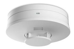
Signal triggering when over 50°C. Permanently installed lithium battery with a service life of at least 10 years. With test button and mute function. Audible alarm with 85 dBA at 3 m. Dismantling safety. Networkable via two-wire line for up to 20 detectors. Networkable via radio module 6828 for up to 20 detectors.
