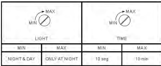
Figure 6: Exploded view of the selection potentiometers for the selection of light and time thresholds.
