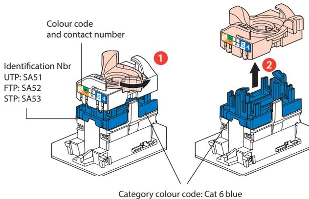
This system allows the wire pairs to be spread easily before mounting them on the connector.
