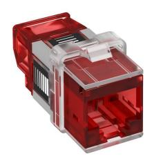
Connection module Cat. 6A (ISO) unshielded, with an RJ45 slot. Including a dust cover, a cable tie, a Keystone fastening frame and mounting instructions. Suitable for installation in the data technology supports of type DTG-2C and DTS-2C, support plate of type MTM 2C and MTM 3C, mounting plate of type MPR2 2C, mounting supports of type MTGE2 2C, MTGE2 15 2C and MTGE2 F 2C.
